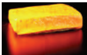
Figure 1. Fabricated brick made of white flour mixed with a small amount of fluorescent powder under UV light (Credit: E. Sisco, M. Staymates/NIST).
