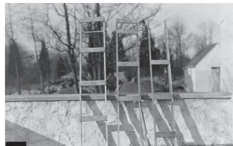
Figure 2. The 3-piece ladder (Courtesy of USDA Forest Products Laboratory: Madison, WI; Forest History Society: Durham, NC).
